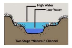
The above diagram provides a good illustration of the two-stage design. The main channel is the lowest part of the stream, and it is meant to hold the normal amount of water running through the stream. A second wider ditch is constructed above the stream. As water rises, the second ditch becomes the main ditch and provides a channel for the high water. Specific dimensions for a ditch is situation dependent.
